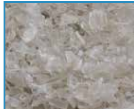
90% PET flake/ 10% recycle flake containing O 2 scavenger
