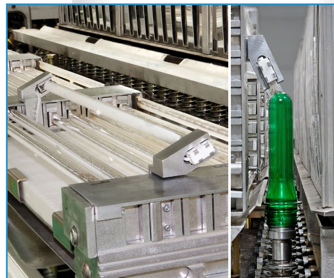
The lamp in a fixed position allows the process to be repeated, faster job change.
